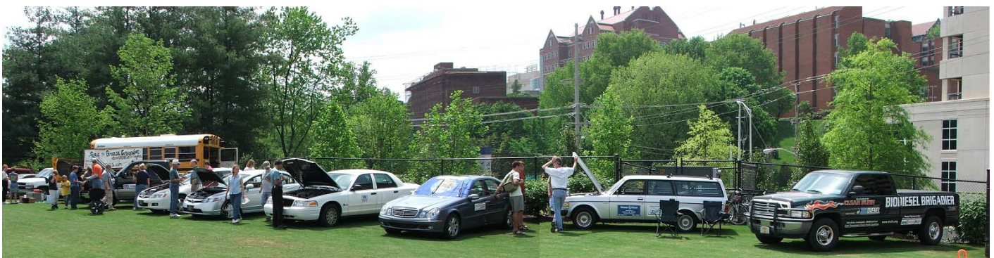
The AFV line-up that the ETCFC showcased during the 2006 Earth Fest (not all AFVs there are shown). Vehicles operating on biodiesel, ethanol, electricity, natural gas and propane were all there, in addition to several hybrids. The school bus at left was running biodiesel but converted to run on straight vegetable oil during the event.
